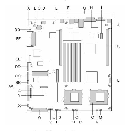
Figure 4: Server Board components
